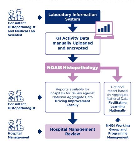
As cases are processed within the laboratory, they are assigned specific procedure codes associated with the type of specimen and quality activities performed. These are recorded within the LIS. Data on all histopathology/cytology cases and the associated quality activities performed are extracted from the LIS and uploaded to NQAIS-Histopathology on a monthly basis by the Local Operational Manager (LOM).
